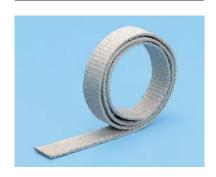
This gasket tape consists of woven glass cloth coated with natural rubber and folded to form a laminated tape.
