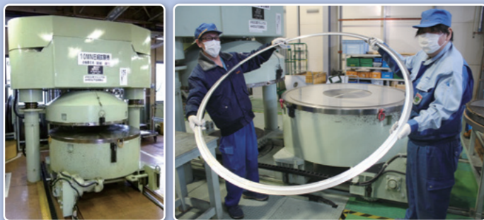
Evaluate the amount of gasket compression required for sealing
